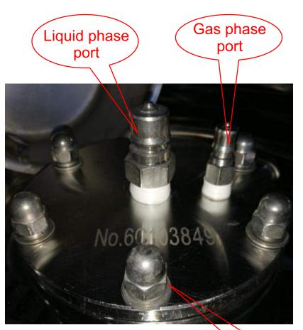
Liquid phase port: In and out for electrolyte, 4P male connector
