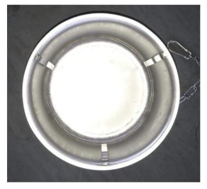
There are fastening screws on the barrel cap. Before use, loosen the screws, then take the barrel cap; After use, cover the barrel cap and tighten the screws.
