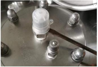
Method 2: 2.1 Insert a scissor under the cap
