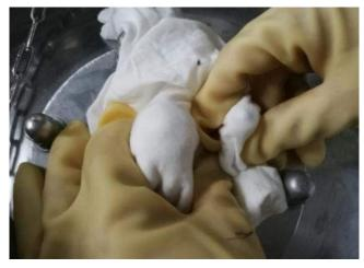
4. After the gas in the barrel is completely out, remove the rags to see whether the leak stops. If not, repeat Step 3 to go on letting out the gas
